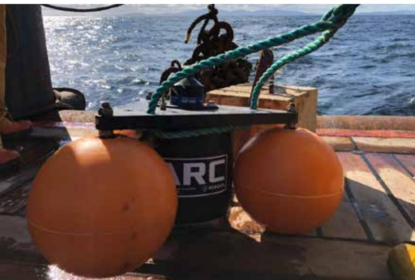
The ARC system is made up of two parts; the upper plate and the rope canister.
