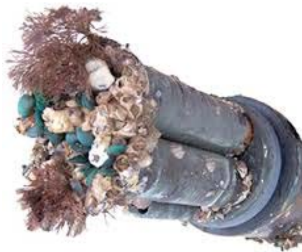
Photo 2 shows a typical multi-sensor configuration. The biofouling occurs at sensor faces where turbulence/flow separation occurs at the interface of the wiper system and sensor areas.
